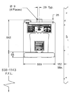
Model SOP50 is our portable eye wash unit. This unit does not require plumbing and is suitable for being wall mounted or placed on a flat surface and includes a stainless steel wall bracket for security. Ideal for low traffic or remote areas where there is the possibility of exposure to injurious or corrosive materials and there is no immediately available supply of portable water.
